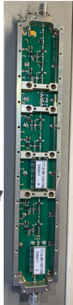
Prototype of 50Ohm LNA (65dB,30-200MHz)
