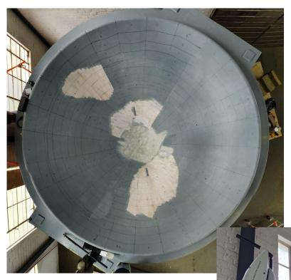
Measurements: Jennifer Studer, Tasmiya Papiah and Keshav Bechoo Plug for forming monolithic dish moulds in Carnarvon, refined and re-characterised after shipping
