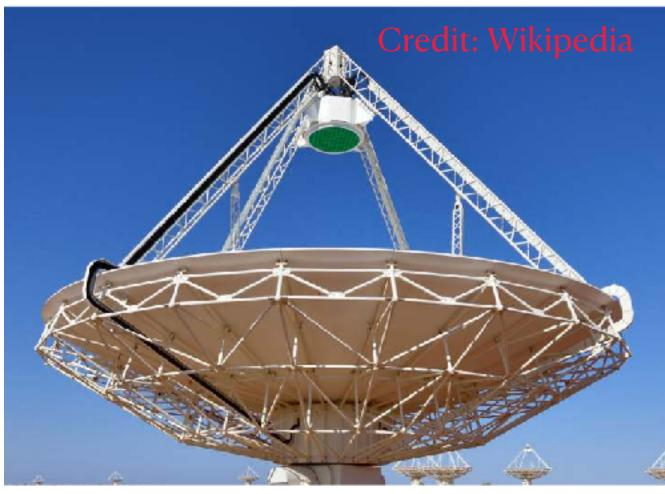
Dimeter :12 m Beam: ~1 deg PAF: ~5.5 deg
