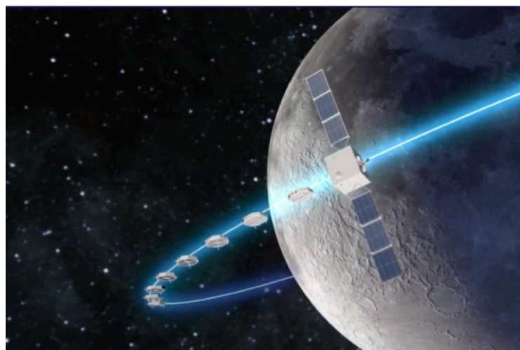
Series (6-8) of tri-pole receivers in lunar orbit to measure the global 21-cm signal and do interferometry
